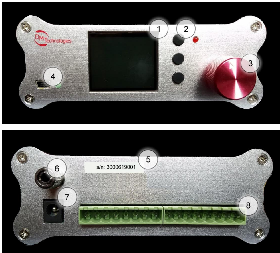
Figure 1. Multichannel current source front (top) and back (bottom) panels.
